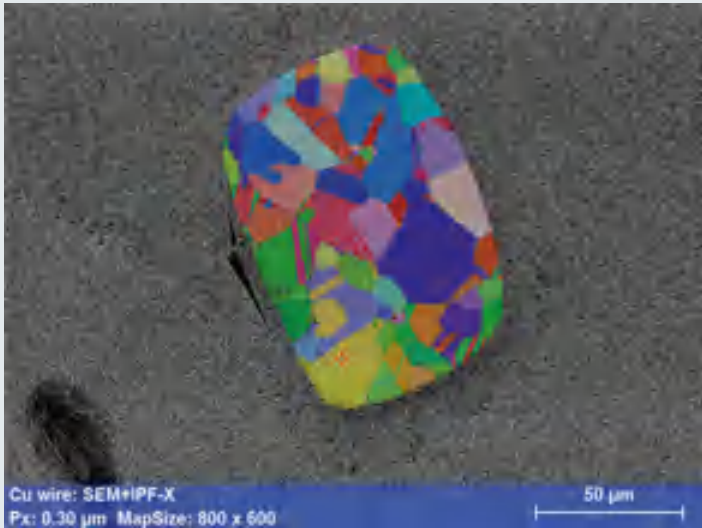
EBSD map of a resin-embedded copper wire
